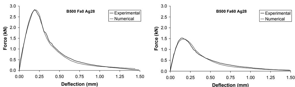
Fig. 5 - Comparison between experimental and numerical  $F-\delta$  curves
