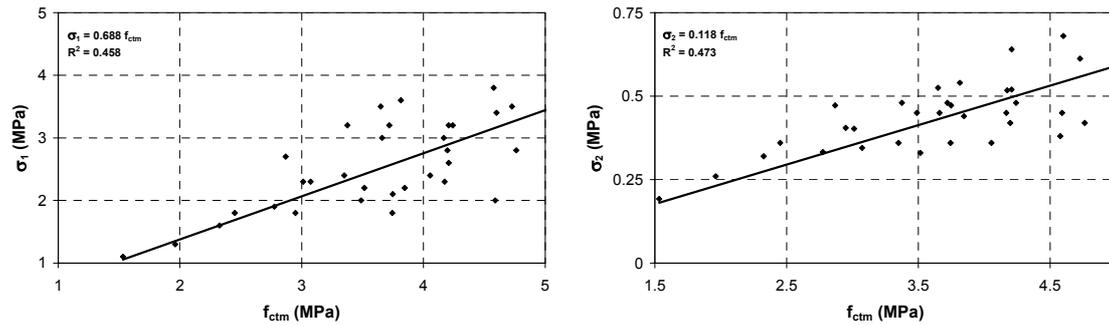
Fig. 14 - Relationships between  $\sigma_1$  and  $\sigma_2$  of the bilinear  $\sigma - w$  diagram obtained from inverse analysis and  $f_{ctm}$  determined from experimental tests
