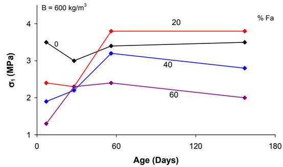
Fig. 10 - Influence of both the specimen's age and the percentage of binder replaced by  $Fa$  on  $\sigma_1$
