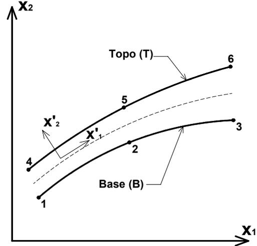
Fig. 1 - Quadratic line interface finite element
