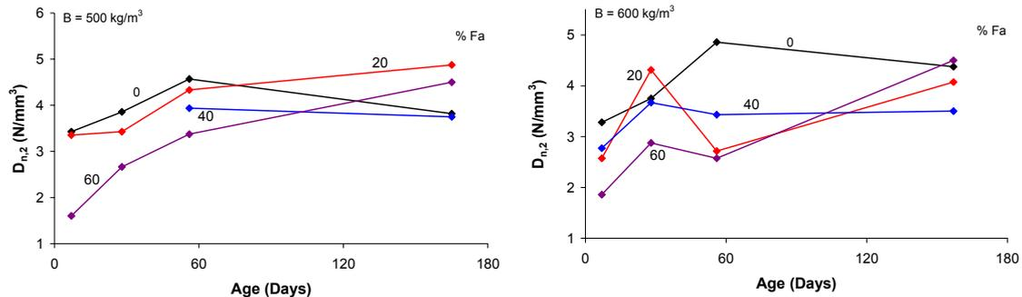
Fig. 13 - Influence of both the specimen's age and the percentage of binder replaced by  $Fa$  on  $D_{n,2}$
