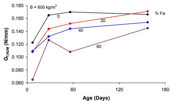
Fig. 9 - Influence of both the specimen's age and the percentage of binder replaced by *Fa* on  $G_{f,NUM}$
