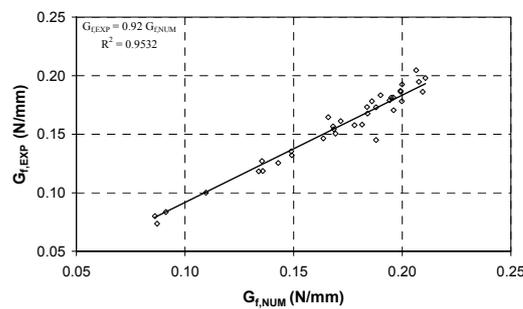
Fig. 8 - Relationship between the fracture energy obtained from numerical and experimental approaches
