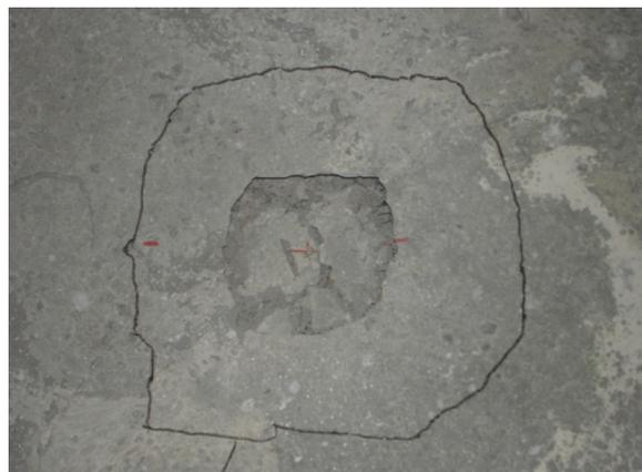
Figure 10. Punching critical contour.
